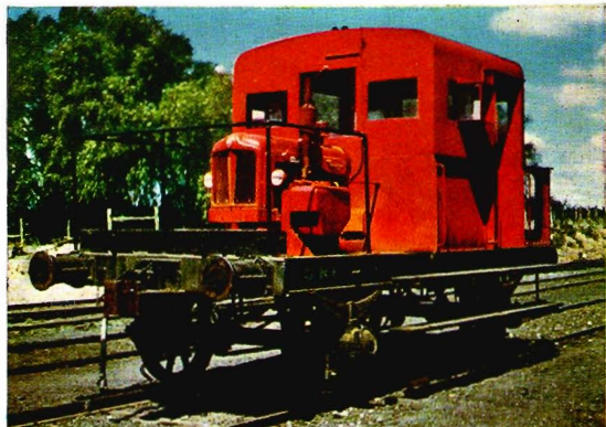
Rail tractor used for shunting in station yards.
