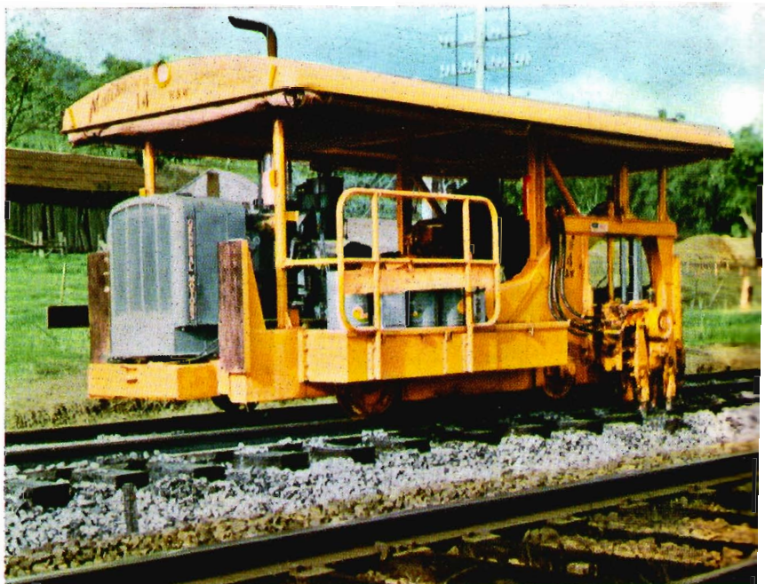
Matisa tie tamper packs the ballast firmly and evenly to ensure a perfect track-bed.
