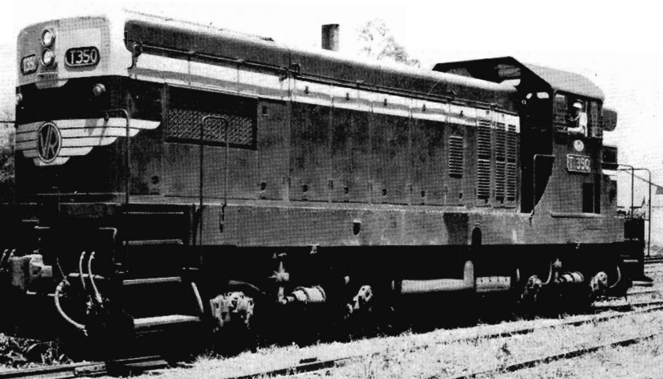
Diesel-electric locomotive, (raised cab roof) 1959 T class
