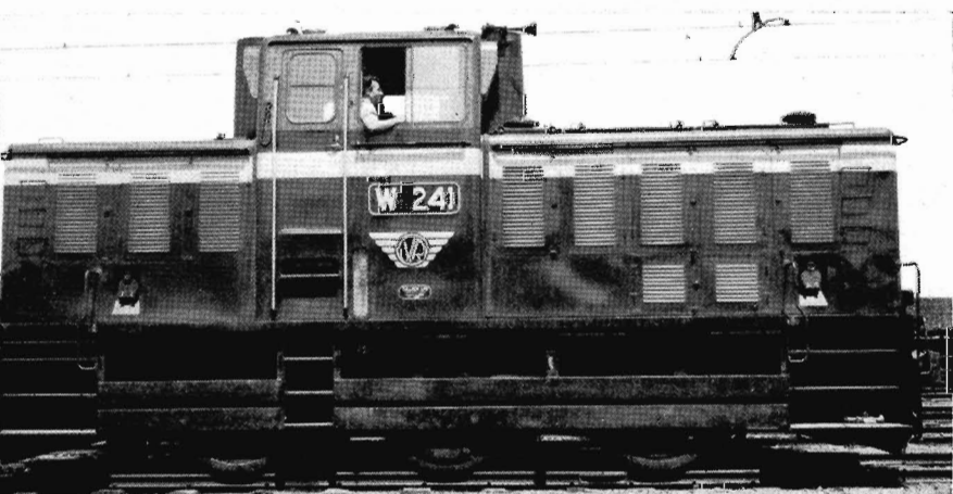
Diesel-hydraulic locomotive, 1959 W class
