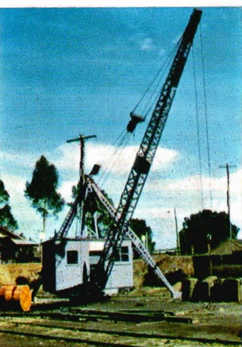
8-ton electric crane at Swan Hill is typical of the specialized equipment installed at various stations to speed loading and unloading of freight.
