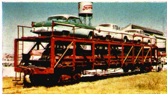
Original double-deck wagon for transporting motor cars from the factory, built 1958.
