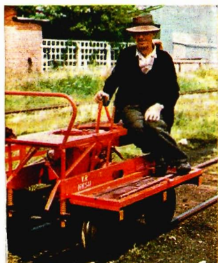
Ganger's track inspection motor, for 2' 6" gauge track.
